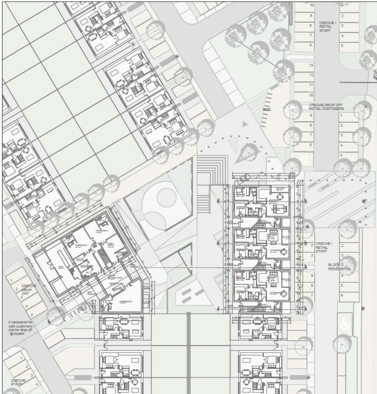
Figure 70.0 Plan excerpt showing the proposed car parking allocation within the neighbourhood centre
